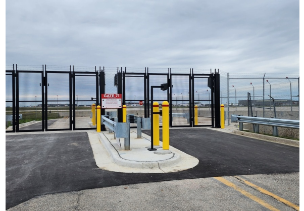
Bi-folding speed gate at a controlled vehicle entry — leaves folded clear of the lane.
