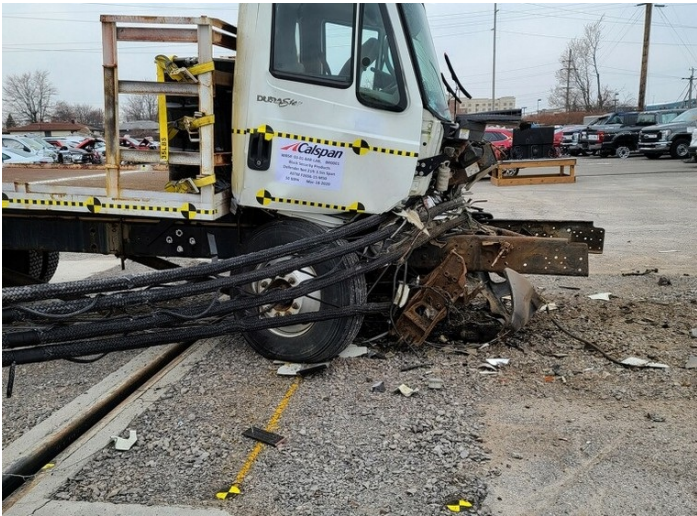
Post-impact at Calspan — the vehicle is stopped and disabled, still held in the net.
