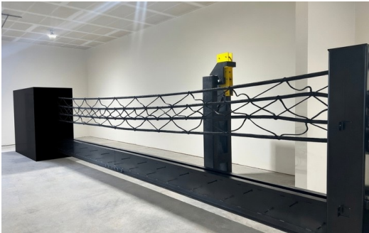
Close up — the four horizontal ropes, the cross-weave that ties them together, and the pan they drop into.
