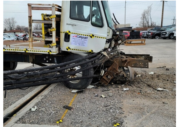
Calspan, after impact — the vehicle is arrested and disabled, the cab intact.
